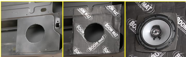
Remove speaker, apply material, re-install speaker
