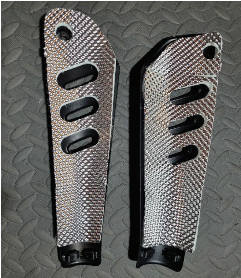
FIG. 2 LAY PIECES INSIDE SHIELD AND PRESS IN PLACE TO FORM THEM TO THE FACTORY HEAT SHIELD
