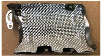
FIG. 8 PRESS BACK INTO THE FACTORY STAINLESS SHIELD. THE SLITS WILLL LINE UP AND YOU CAN BEND IT TO A SNUG FIT
