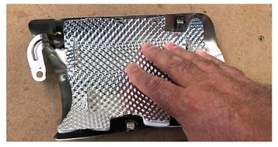
FIG. 6 LAY GLASS FIBER IN CAT SHIELD THEN ALUMINUM SHIELD ON TOP AND PRESS DOWN ADN FORM THE TWO PIECES TO THE CAT SHIELD.
