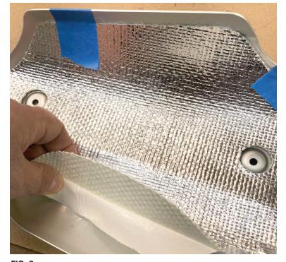
FIG. 3 USE TAPE TO HOLD SHILED INTO PLACE AND START TO PULL BACK RELEASE LINER.
