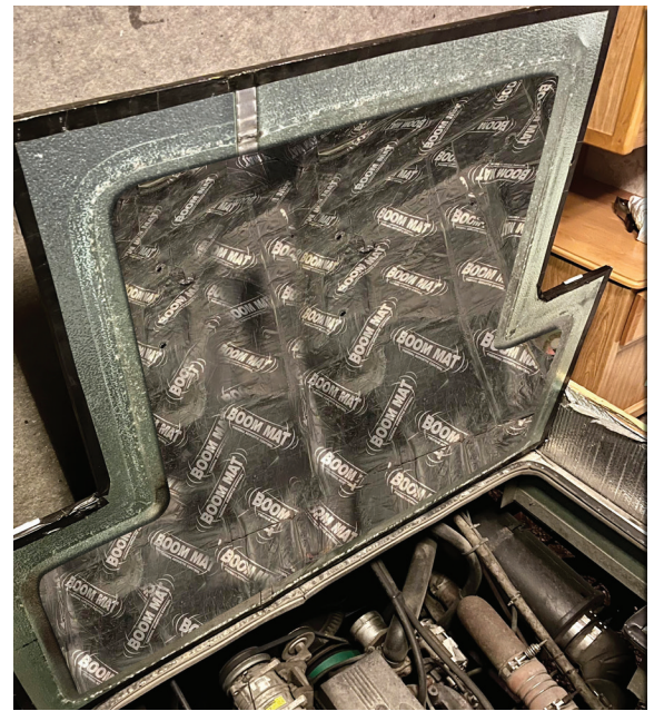
Damping material installed on under side of engine cover
