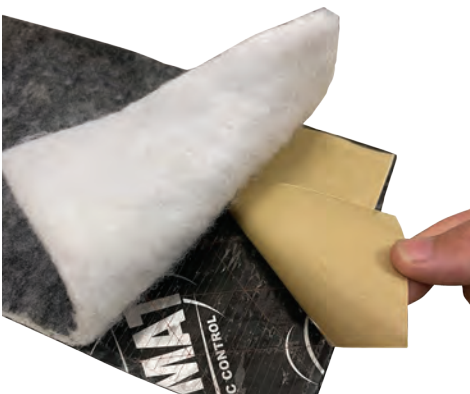
FIG. 4 Install strips of adhesive Transfer Tape to the floor pan where needed to hold Under Carpet Lite insulation in place. The placement is not critical. Just apply to areas to hold insulation in place. Once applied, peel back liner of tape and press Under Carpet Lite Insulation in place.
