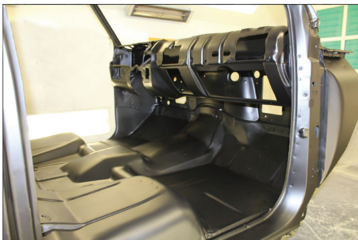
FIG. 1 Remove seats, console & carpet. Clean dirt/debris and recommend using sealer on any rust spots (View from passenger side)
