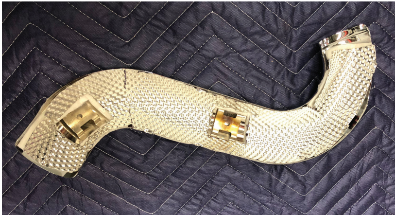
FIG. 17 PRESS LINER INTO SHIELD
