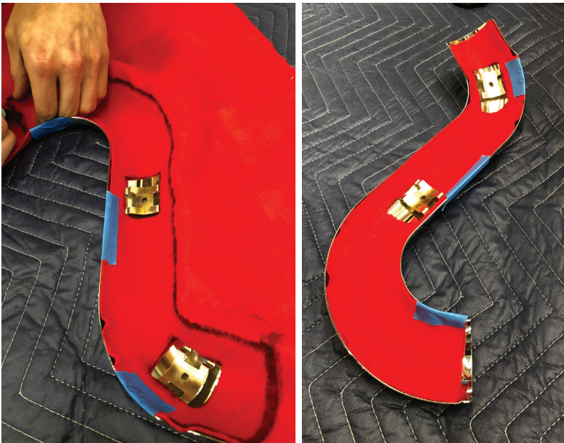
FIG. 8 TRACE THE REST OF THE SHIELD AND CUT OUT WITH SCISSORS
