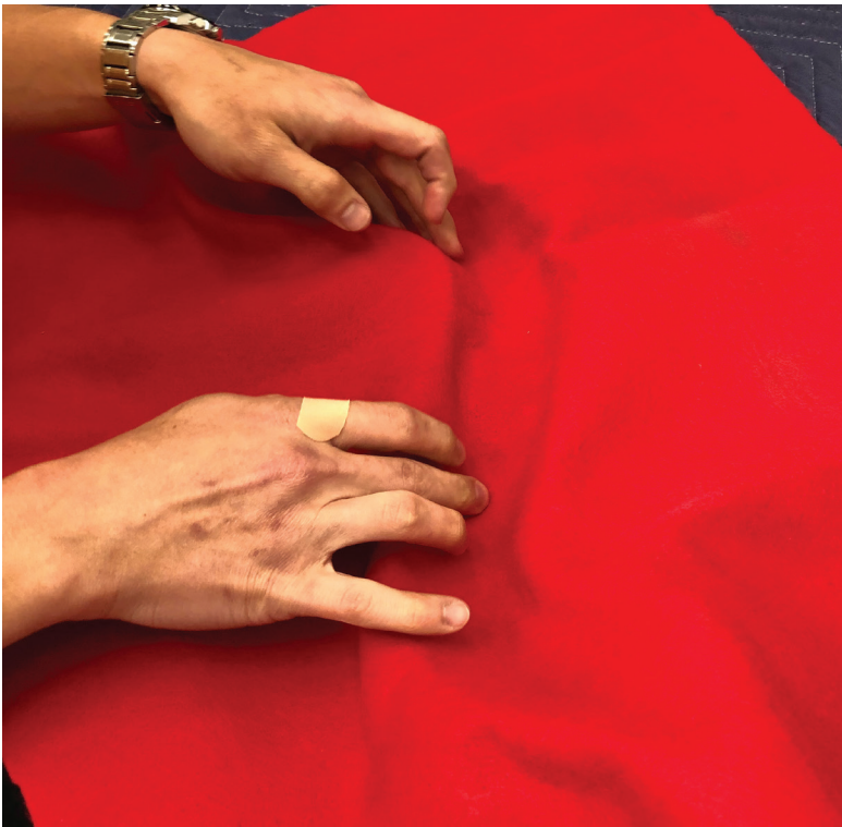
FIG. 2 LAY FELT OVER SHIELD AND PRESS IT INTO THE BACK OF THE SHIELD
