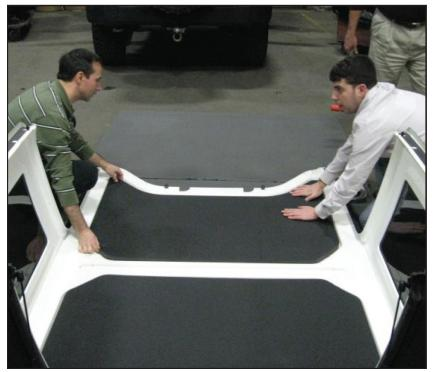
5.) Once the starting edge is adhered, lay down the rest of the part by applying gentle pressure by hand as shown in Figure 4.
