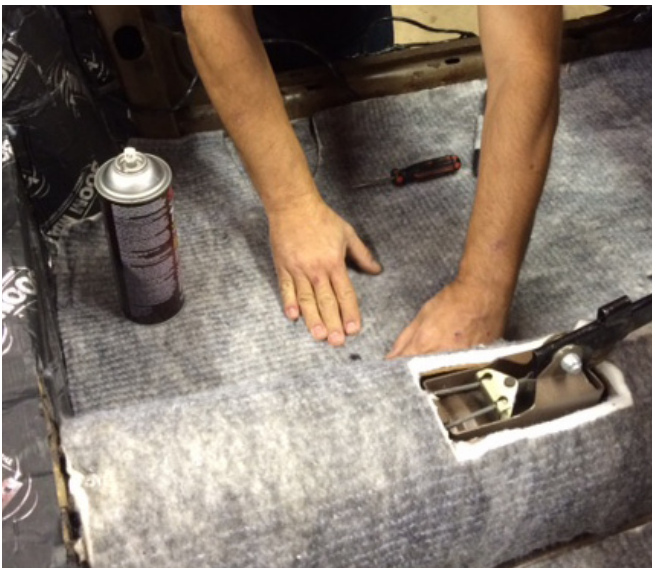
UC Lite trimmed and being applied with spray adhesive.
