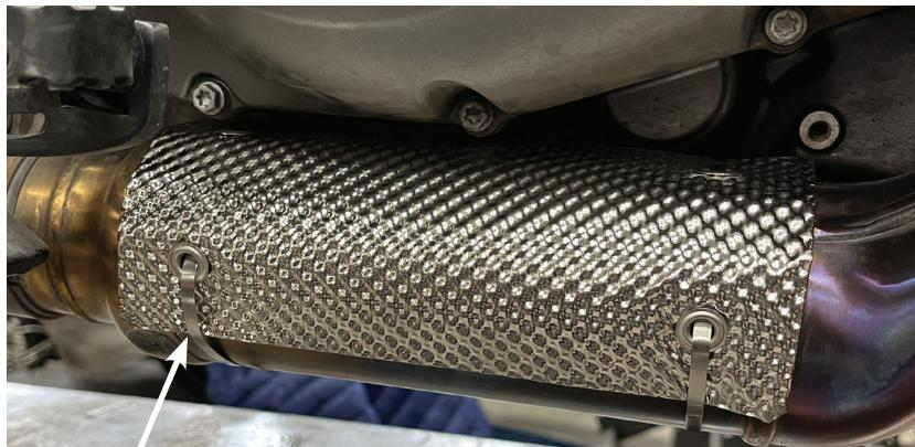
**FIG 5** Route ties over and behind catalytic converter and start ties.
