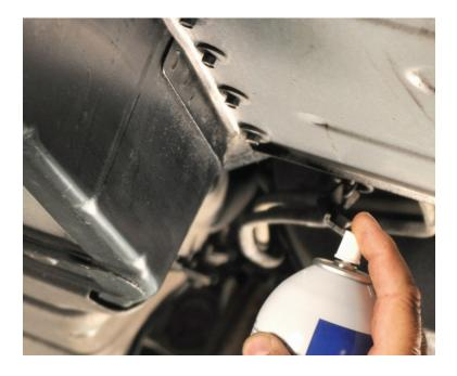
NOTE: It is very important to clean the area where the pieces will be adhered and make sure it is free of grease, oil and dirt.
