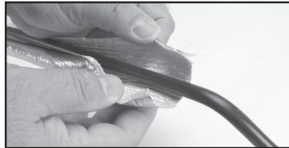
STEP 3. As you wrap the line, peel back the adhesive backing & fold over the adhesive flap pressing down to close the sleeve.
