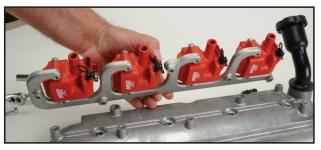
STEP 1. The heat shields are the same for either side.
