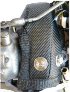
anchor point. Anchor point style may vary depending on your particular turbo shield. (Fig 2, Fig 3, Fig 4)
