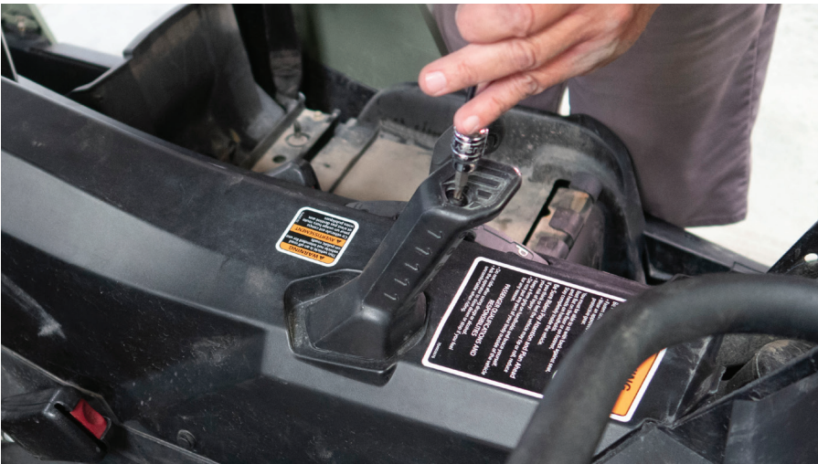
Fig. 2 - Remove Torx screws from handles and slide rubber grips up and off
