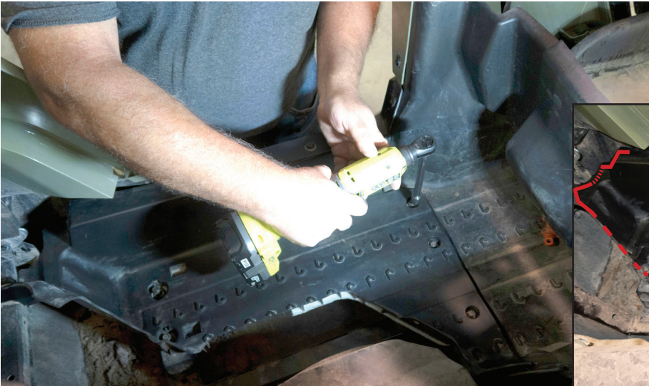
Fig. 14 - Remove rear driver side floor panel
