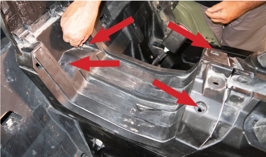
Fig. 1 - Remove push pins from entire perimeter of console. You can use tool as shown to the right, or a flat head screw driver to pop up the center of the push pin, then pull it out of the hole
