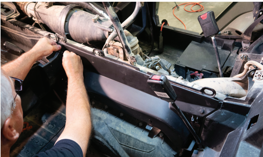
Fig. 12 - Remove rear center consol side panel
