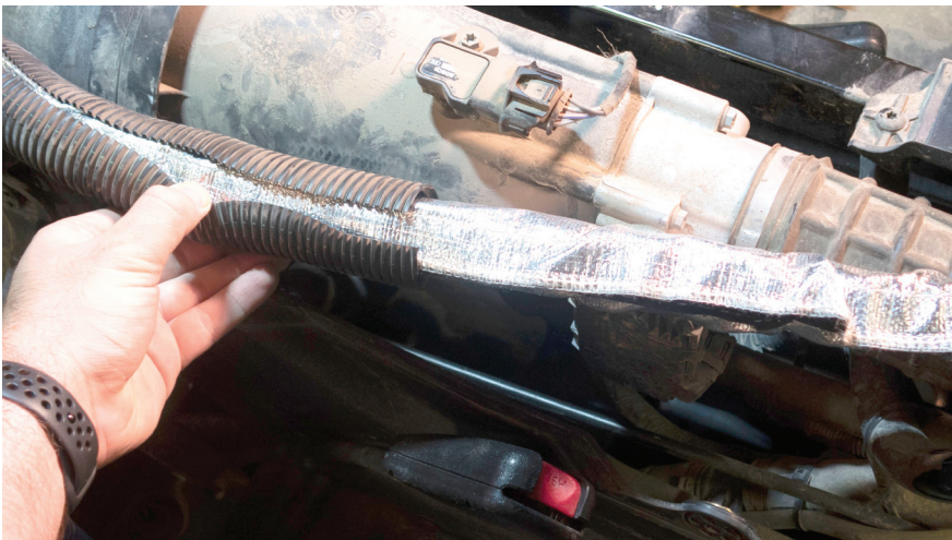
Fig. 18 - Peel back plastic tubing on coolant line and install Heat Shroud reflective sleeve
