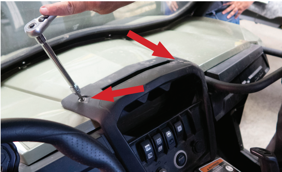
Fig. 4 - Remove Torx screws from top of center dash
