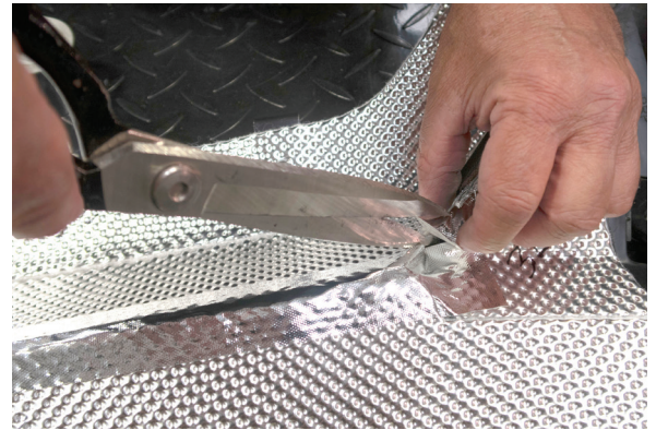
Fig. 21 making small relief cuts helps when installing Cool Tape around bends and curves
