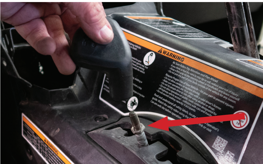
Fig. 3 - Loosen jam nut (red arrow pointing at jam nut) and unscrew shifter knob
