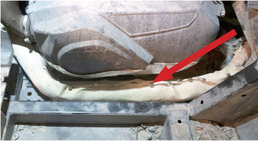
Fig. 16 - Wrap exhaust wrap material around front header pipe and secure with provided speed clamps
