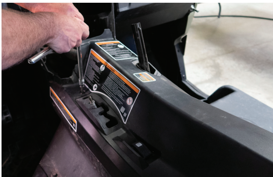
Fig. 6 - Remove main console fasteners on driver side and lift up to unplug override switch
