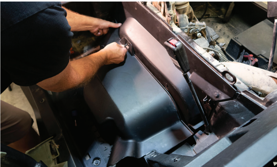
Fig. 11 - Remove rear driver side floor piece
