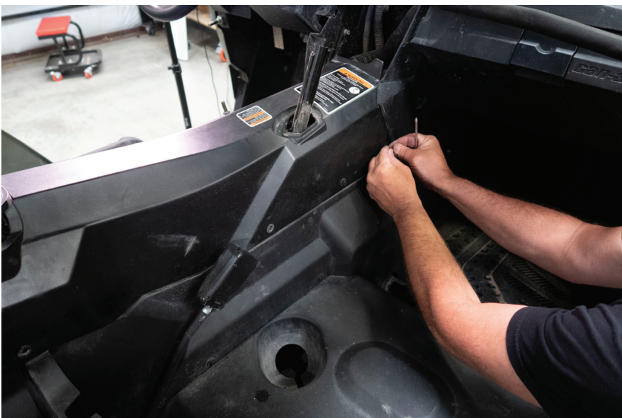
Fig. 9 - Remove remaining center console fasteners
