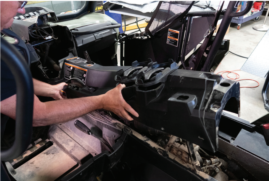
Fig. 10 - Remove center console by lifting up and ahead to clear grab handle bars
