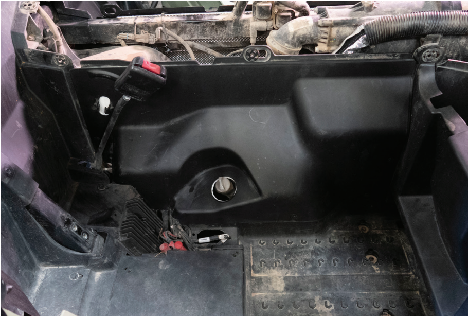
Fig. 13 - Remove passenger side rear center console trim. (Piece with oil fill opening in it)
