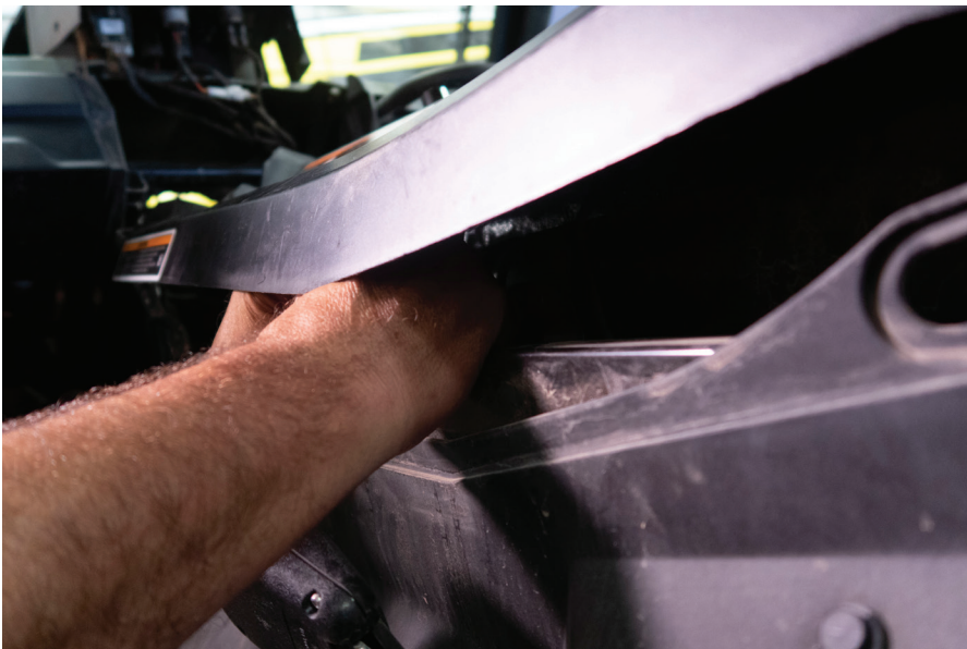
Fig. 7 - Lift up slightly and unplug Override switch
