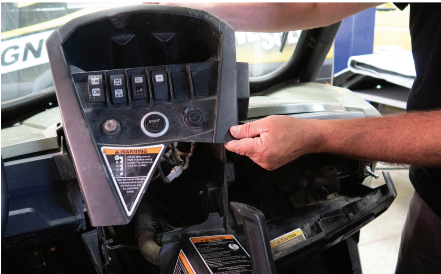
Fig. 5 - Open glove box door, lift center console back and up. Set on dash with wiring connected.
