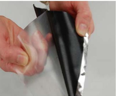
2. Remove the release liner to expose the adhesive.
