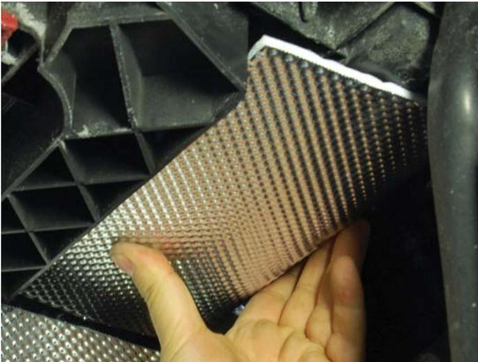
23. Before peeling the protective backing film, pre-fit the shield by sliding it from the bottom of the battery box up the side and bending the bottom 90 degrees until it meets the edge of the box. (Image K)
