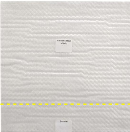
14. Locate the Heat Shield marked (Harness Heat Shield) (Image G). The bottom portion of the protective backing film has been pre-cut. This will attach to the fire wall just below the harness connectors.
