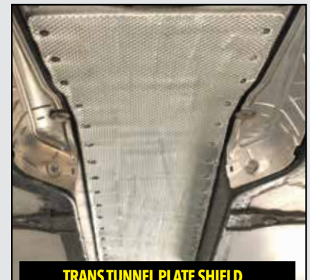
TRANS TUNNEL PLATE SHIELD
