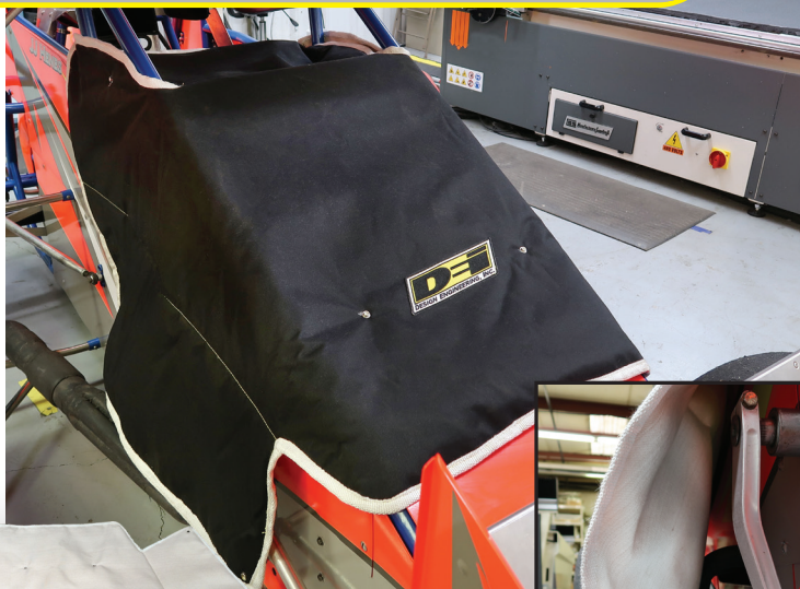
HIGH-TEMP FIBERGLASS PANELS CAN REST DIRECTLY ON HEADERS
